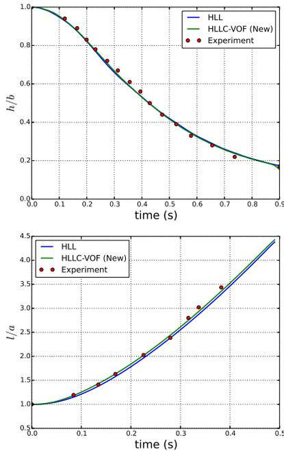
Figure 3: Dam break - height and surge position
