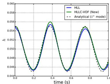
Figure 5: Low amplitude sloshing - first mode
