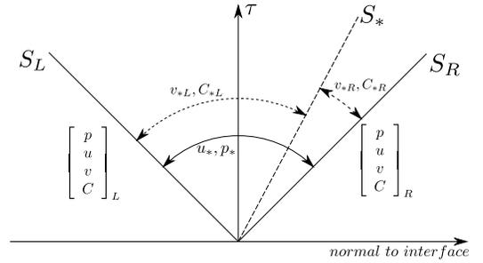
Figure 1: HLLC-VOF wave structure
